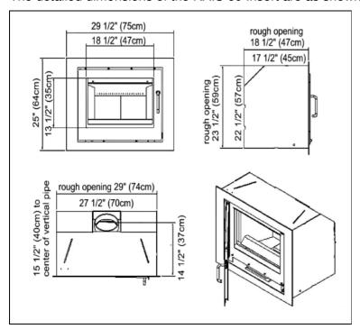
Although the RAIS 60 Insert comes assembled, it has to be mounted into the fireplace or firebox.
