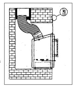
Fire stops must be installed at spaces where the chimney passes through floors and/or ceilings.
